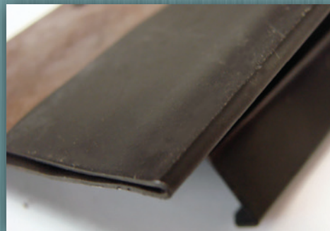
STRYK 5388 FACS® applied on Q-panel 10 Mils Dft folded 180 degrees
